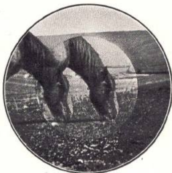
FIG. B— LEICA out of focus . . . Double image is conveniently within the LEICA range finder field of view.
