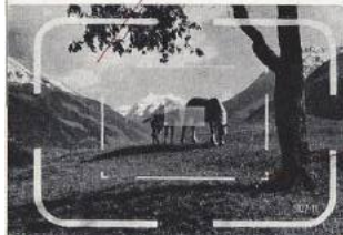
Field of view with a 90 mm LEICA lens. The subject area covered with the longer focal length is indicated by the additional bright line frame within the large brilliant frame showing the field of view of the 50 mm lens, which remains visible all the time.
