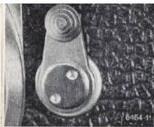
Lever in normal position: field of view for 50 mm lens
