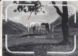
Field of view with the 135 mm HEKTOR lens which yields a magnification of 2.7 times as compared with the standard 50 mm lens.
