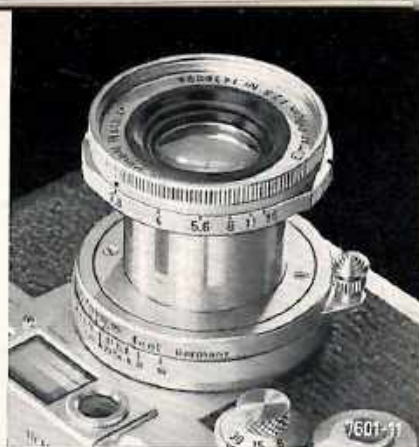
Lens locked at "infinity".
